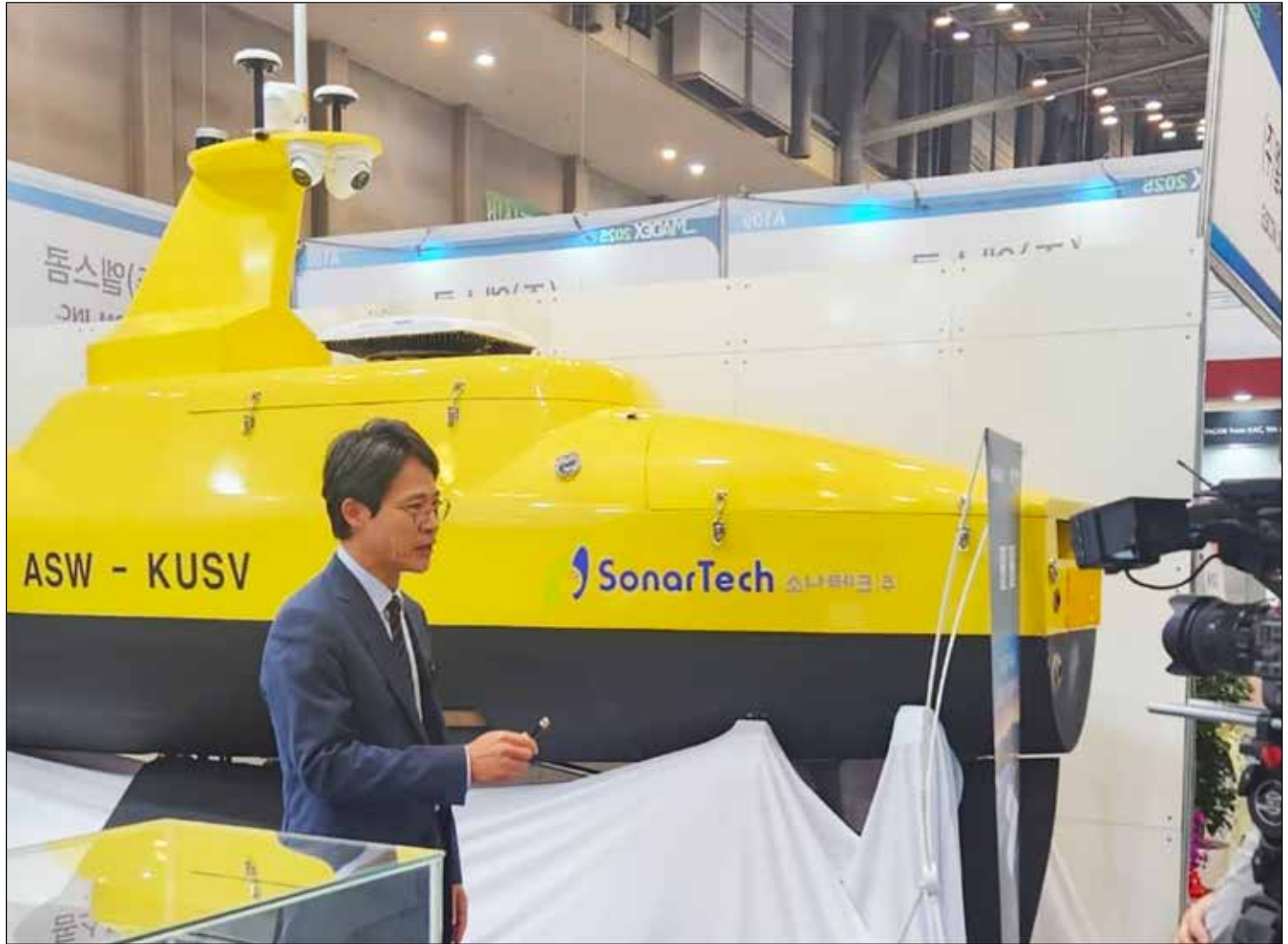
South Korea's 20-ton twin-sonar sea drone turns oceans into sub hunting grounds. (Photo: SonarTech.)
